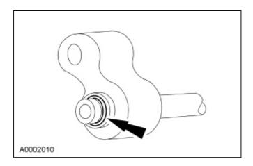
3. **NOTE:** When correctly assembled, the male and female fittings should be flush.
