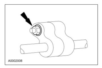
2. *NOTICE:* Do not use metal tools to remove the O-ring seal. They can cause axial scratches across the O-ring seal groove, resulting in refrigerant leaks.
